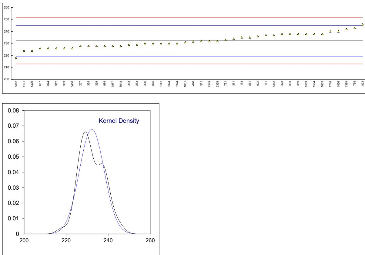
Determination of Kinematic Viscosity at 40 °C on sample #22075; results in mm<sup>2</sup>/s
