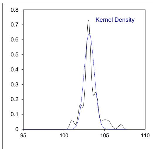
Determination of Kinematic Viscosity Stabinger at 40 °C on sample #22075; results in mm<sup>2</sup>/s
